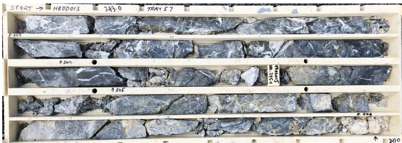
Figure 5: Intense silica-sericite-pyrite alteration in the 650 Zone (half-NQ core, 243m-247m).
