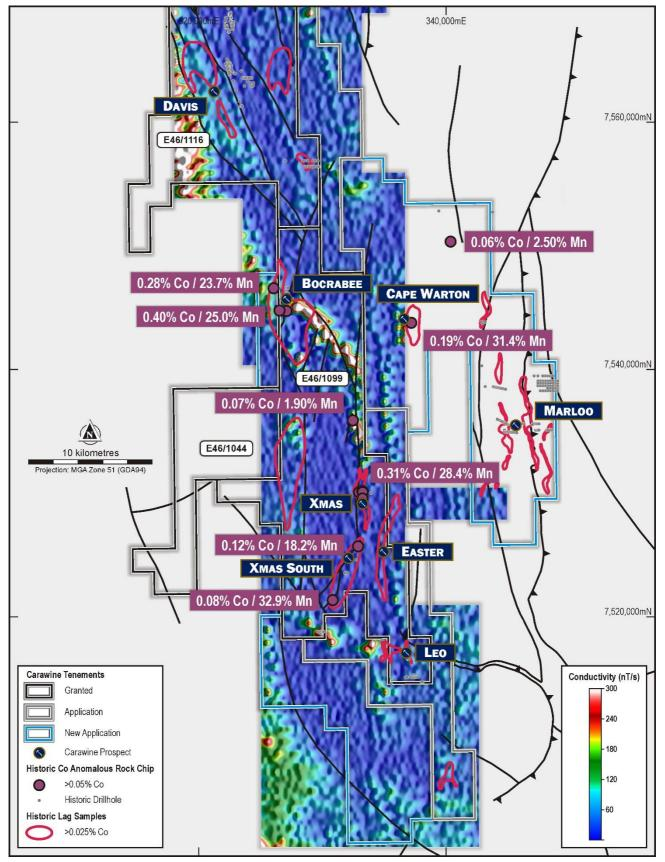
Figure 2: CRAE GEOTEM survey conductivity image channel 15 and regional cobalt-manganese targets.
