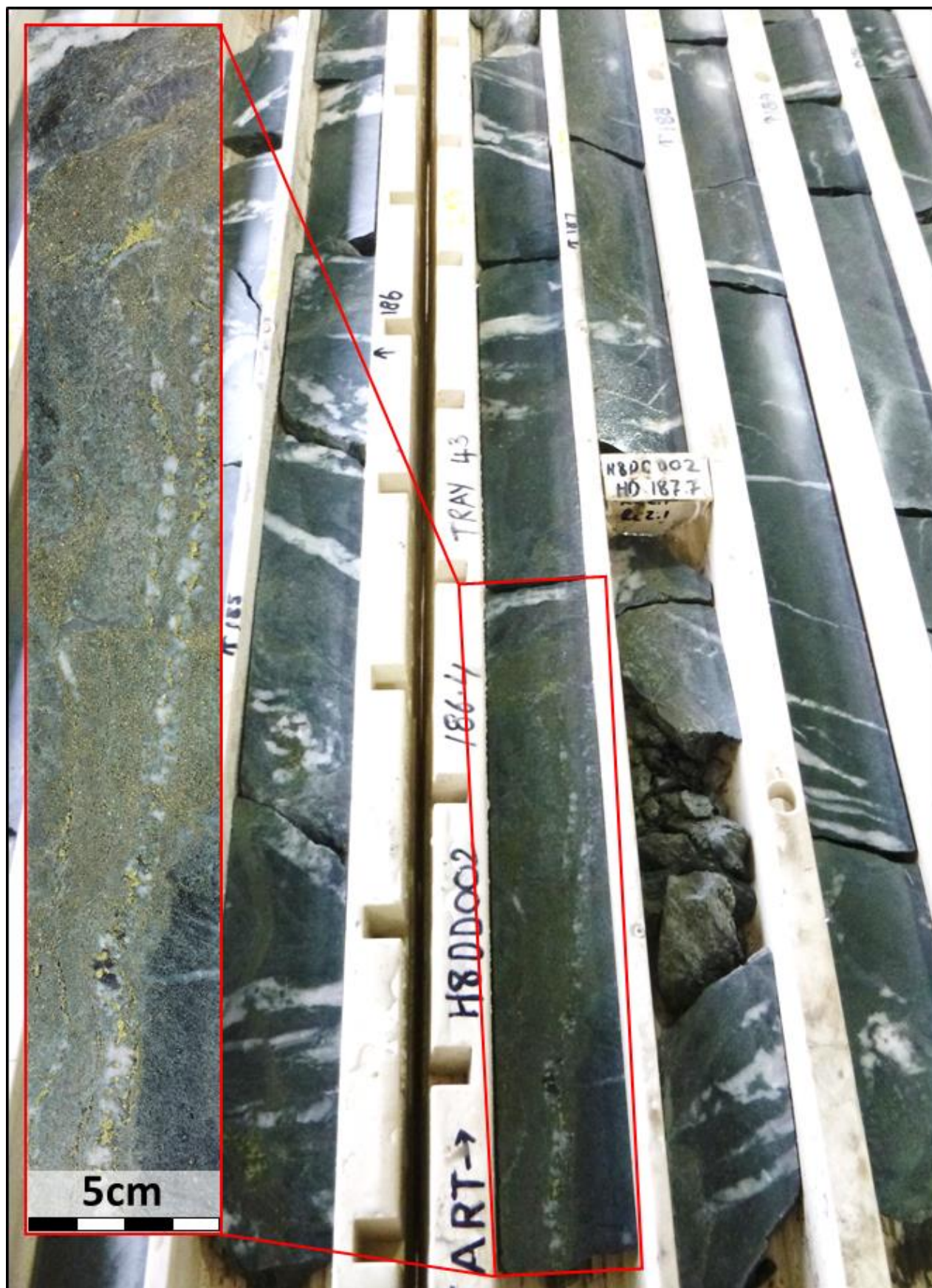
Figure 3: H8DD002 stringer zone mineralisation with quartz-chalcopyrite veining and chlorite-dominant alteration (half NQ core, inset 186.4-186.7m downhole).
