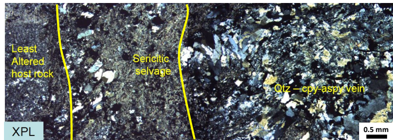
Thin section – sericitic selvage to qtz-cpy-asp vein (XPL)
