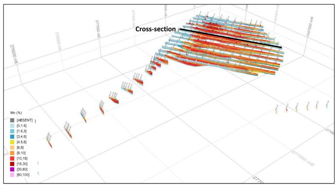
Figure 6. Oblique view of the FB3 Mineral Resource model looking northeast and coloured by Mn grade (%) (2x vertical exaggeration). (Labels represent drill holes used in the estimate)
