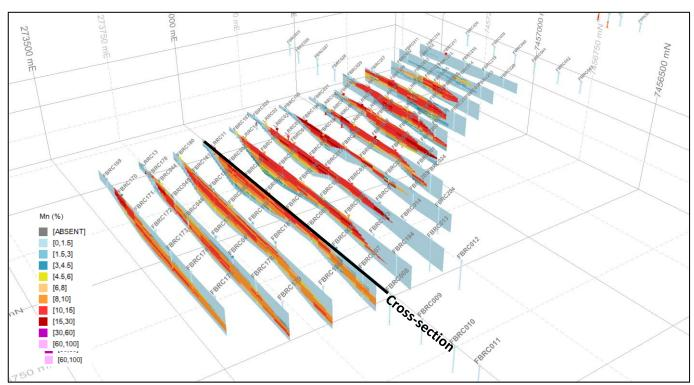
Figure 8. Oblique view of the LR1 updated Mineral Resource model coloured by Mn grade (%) (2x vertical exaggeration). Labels ("LRRC01-22) represent historic drillholes used in the estimate)
