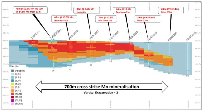
Figure 9. Type section 273,760 mE (looking east) showing LR1 Mineral Resource model cells and drill holes coloured by Mn grade (%) (2x vertical exaggeration)
