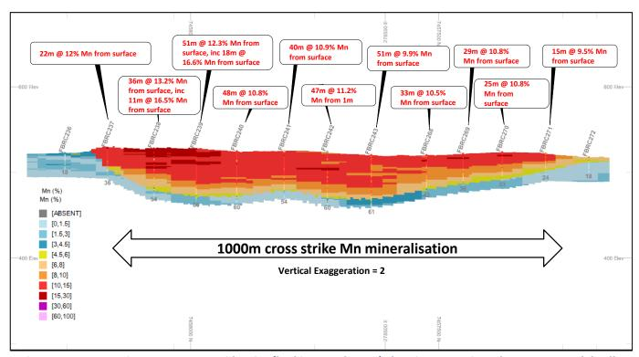
Figure 7. Type section 278,430 mE mid-point (looking north-east) showing FB3 Mineral Resource model cells and drill holes coloured by Mn grade (%) (2x vertical exaggeration)
