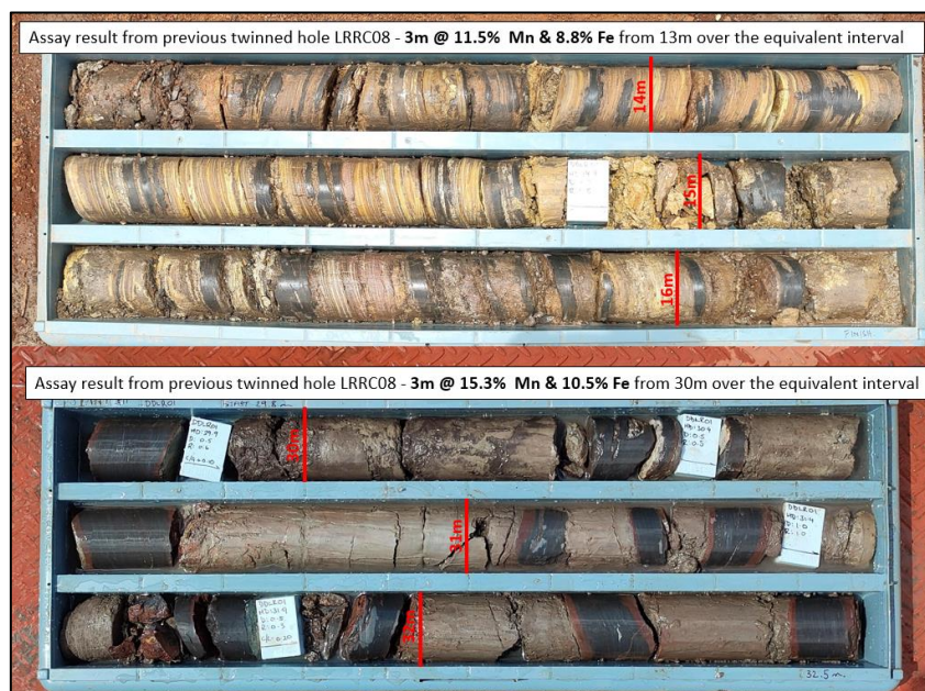
Figure 1. Recently drilled Black Canyon diamond core hole DDLR01 that is twinning historic RC hole LRRC08 that intersected 37m @ 12.8% Mn and 10.5% Fe from 3m 3 . Manganese bands are dark grey in colour. Note that the assays quoted are from the equivalent interval in historic drill hole LRRC08 and assays for DDLR01 are pending.
