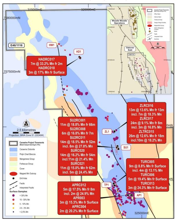
Figure 2. Fig Tree Manganese prospects and significant previous drill results
