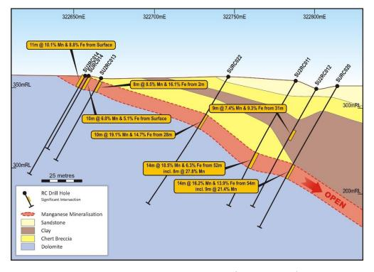
Figure 4. SU1 prospect Cross section (looking north)
