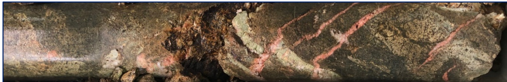
Potassic veining, alteration and boxworks after sulphide (H8DD023, 80.5m, NQ core).
