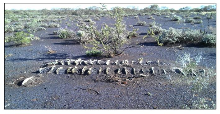
Figure 10. Drill rig spoil from historic drill hole LRRC03 (EOH 42) with samples laid in rows of 20m
