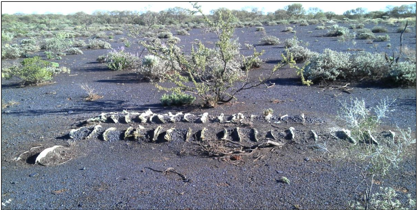
Figure 6. Drill rig spoil from hole LRRC03 (EOH 42) with samples laid in 20m columns
