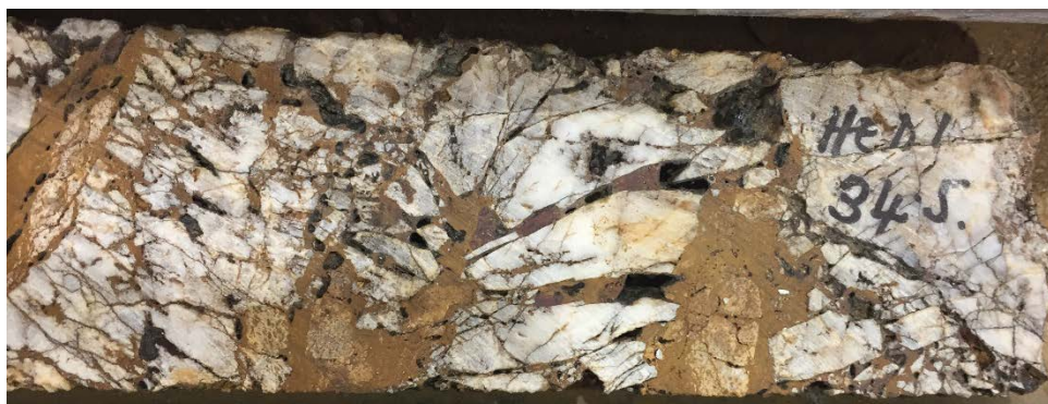
Quartz-carbonate-sulphide breccia from 34.5m in drill hole HED1 (half-HQ core)
